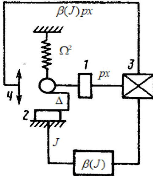
**Fig. 1.** Example of a system with one degree of freedom: 1 - speed sensor; 2 - impact impulses sensor; 3- signals multiplier; 4 – vibration exciter.
