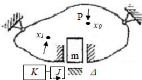
**Fig. 1.** General view of the studied mechatronic vibro-impact system
