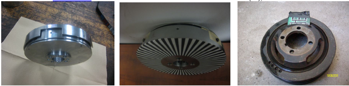
Figure 13. Prototypes of different versions of Tuned TVD
