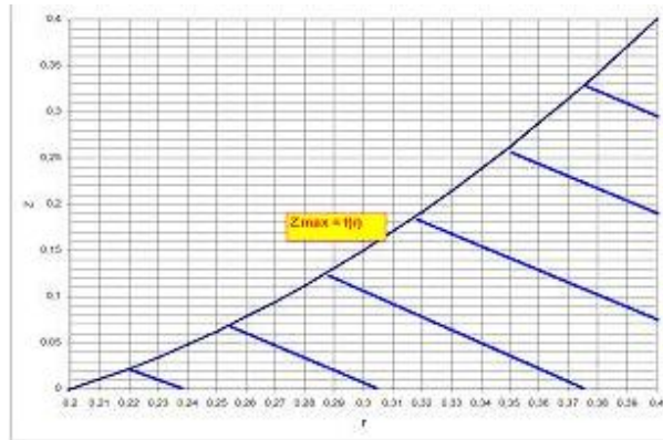
Figure 6. Selection of the constant deflection of a spring beam of TVD
